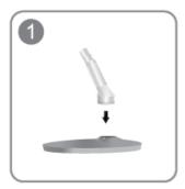
Insert the Stand Connector into the Stand Base in the direction shown by the figure.
